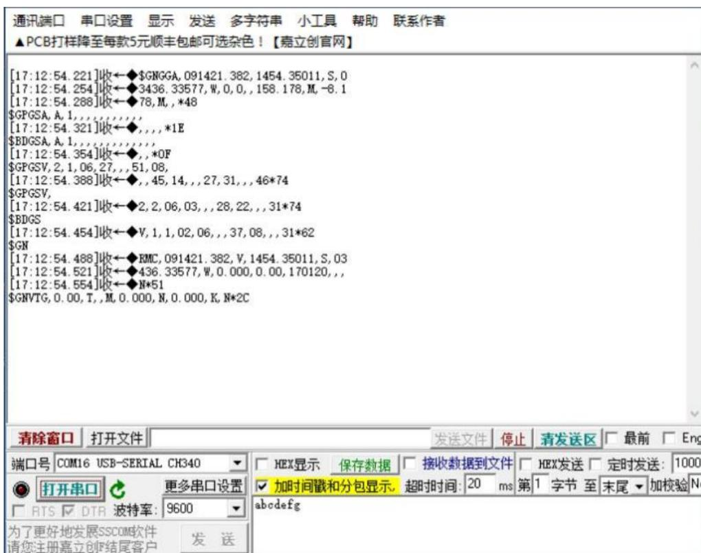
the baud rate is set to 9600bps and the serial port is opened, data will be reported continuously. The common output format is as follows:
