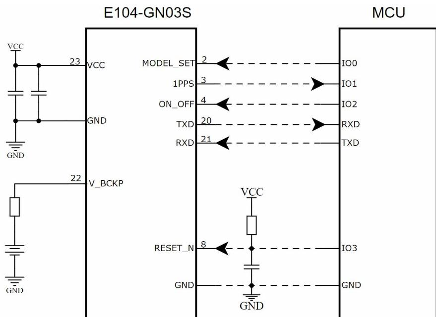
The battery charging current limiting resistor needs to be adjusted according to the battery parameters. A  $200\Omega$  resistor is connected in series inside the module.
