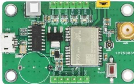
After connecting the GPS antenna, connect it to the computer via a USB cable. There is a USB port on the opposite side of the antenna on the board . Then press the power button to turn it on.
